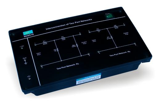
Interconnection of Two Port Networks, NV6519 has been designed specifically to demonstrate the importance of Interconnection of Two Port Networks. It can be used as a stand alone unit with inbuilt DC power supply.
