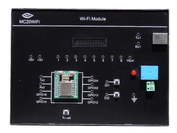
MC20WiFi Modules is an extension module for Nvis Microcontroller development platforms. The module has been designed for students and practicing engineers to gain invaluable practical experience on the principle and applications of microcontroller & Wi-Fi module. The object is to have a clear understanding of how Wi-Fi module is interfaced and controlled with microcontroller and PC. Wi-Fi modules are embedded solutions providing wireless end-point connectivity to devices.
