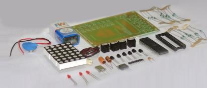
Binary to Dot Matrix Display is based on 8051 microcontroller family, it shows conversion of binary number to hexadecimal number on dot matrix display. The circuit is powered by 9V battery source. Four switches are used to select the sixteen binary combinations (0000 to 1111).
