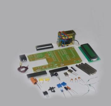
In this circuit, microcontroller AT89C52 counts and shows on an LCD the number of interruption made between IR transmitter and receiver. The IR transmitter (IR LED) generates 38 KHz frequency from 555 timer. At receiver this frequency is sensed by IR receiver IC TSOP 1738. The interruptions generate pulses which are counted by the microcontroller and then display the counts (number of interruption) on LCD.
