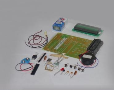
Nvis 33D is a versatile security device based on microcontroller 8051 family, which gives the alternative of keys. The user can set a 3 digit password (000-999). Light and sound indications are given for correct / incorrect passwords. User has 3 chances to enter passwords. The circuit is operated using 9V battery
