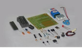
Nvis32D Bidirectional visitor counter is a circuit used to show the number of people entering & leaving a room. To demonstrate this, the user can use any opaque object to cut link between the two IR pairs. Depending on the direction of movement the display is either incremented or decremented.
