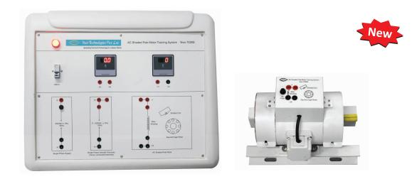
AC Shaded Pole Motor Training System is an exclusive training system for electrical laboratories. It provides complete learning contents and students can easily understand the fundamental concepts of AC Shaded Pole Motor. AC Shaded Pole Motor having poor torque at load condition and so this motor majorly used in small appliance such as hairdryers, polishers, blowers, etc.
