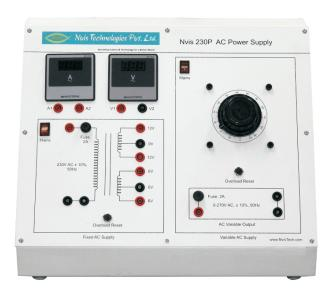
**Nvis 230P "AC Power Supply"** is a versatile product mainly used in electrical and electronic engineering laboratories for the purpose of conducting experiments over AC circuits. This unit provides 0-220V Variable AC output and 6V-0-6V & 12V-0-12V step down AC Voltage with adequate protection schemes. Digital voltmeter and ammeter are being used for better resolution and accuracy.
