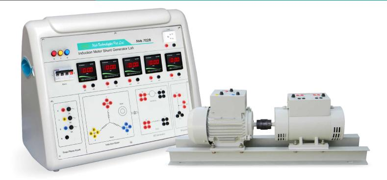
**Nvis 7028 Induction Motor Shunt Generator Lab** is a significant training system for Electrical Machine Laboratories to demonstrate the operational working and characteristic of DC Shunt Generator under different loading conditions. DC Shunt Generator is a type of Generator whose field winding and armature winding are connected in parallel and acquire properties to behave as almost constant speed DC Machine.
