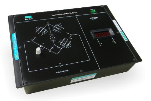
**Nvis 6534 Experimentation with Kelvin's Bridge** is a useful training product for measuring very small values of resistance. Kelvin's double bridge or Kelvin's bridge (as it is commonly known) is a variation of Wheatstone bridge and is based on the same principle. By setting the null point we can evaluate the unknown resistance. This product has Digital Display (DPM) for the purpose of null detection implemented on the trainer board itself.
