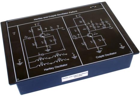
**Nvis 6505 Experimentation with Hartley and Colpitt Oscilllator** is an elite training system for the analog electronics laboratories. It is useful in understanding the basic concepts and functioning of both Hartley and Colpitt Oscillators, and their use in generation of Sinusoidal Waveform.
