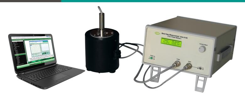
**Nvis 6105 Resistivity and Band Gap Measurement of Semiconductor** is a versatile and useful training system for Physics and basic Electronics laboratories. In Nvis 6105, Band Gap can be measured by using Four Probe method.
