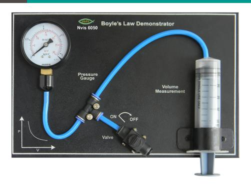
**Nvis 6050 Boyle's Law Demonstrator** helps students to understand the relation between Pressure and Volume. Gas laws are basic laws that give the relation between the three basic properties of gas like Temperature, Pressure and Volume.
