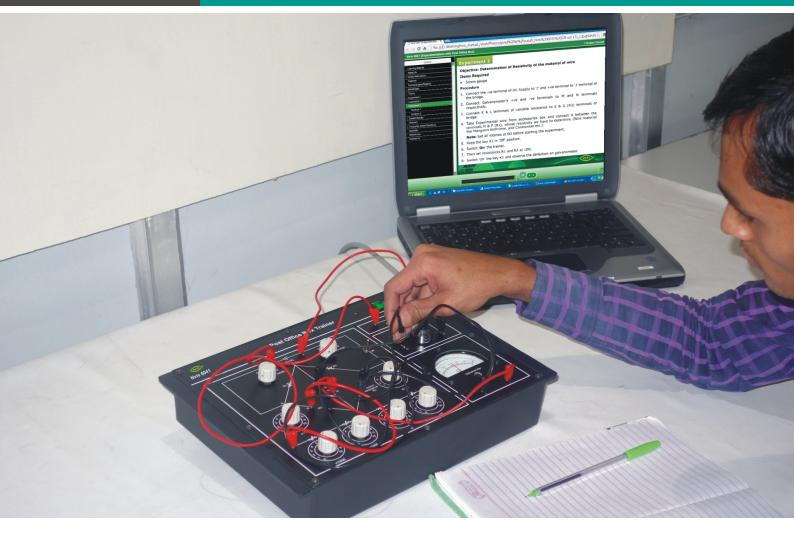
Nvis 6041 Post Office Box Platform is the combination of resistances which work on the principle of Wheatstone Bridge. Post Office Box is helpful to determine the unknown resistance of wires like Constantan, and Nichrome etc. With the help of Nvis 6041 we can determine the specific resistance of different types of wire. Post Office Box can also verify the combination of resistance in series and parallel.
