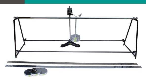
**Nvis 6040 Young's Modulus Setup** is a complete system used to determine Young's Modulus of Elasticity of materials. When a metal wire is stretched beyond its elastic limit then its cross section is reduced i.e. its structure is changed internally. These changes increase with repeated drawings. The hardness and elasticity of the material are profoundly affected. Setup is used to investigate the change in length of a sample under a varying tension.
