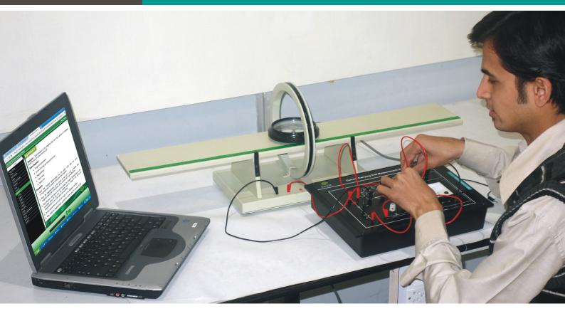
**Nvis 6034 Current Carrying Coil Setup** is designed to explain the concept of Electromagnetism. This product is also known as Stewart and Gee's apparatus. This setup is helpful for the study of magnetic field around a current carrying coil. It illustrates how magnetic field is generated by applying electric current in any current carrying conductor. For this purpose Tangent Galvanometer is used, which is based on Tangent law of magnetism.
