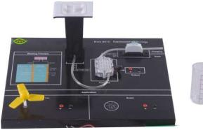
**Nvis 6013 Experimentation with Bio Energy** is used to demonstrate the functions of renewable fuel cell using Isopropylalcohol as the biofuel.
