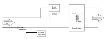
For understanding the role of Relays in real time transmission system, a circuit of transmission line is provided from source to distribution with proper placing of all its components
