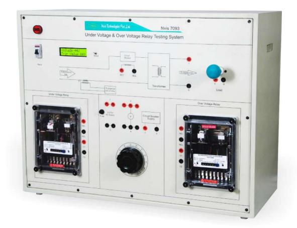
**Nvis 7093 Under Voltage & Over Voltage Relay Testing System** is intended for advanced practical training in protective devices connected with transmission lines, cables and network sections in power systems lab. A Relay is an electrically operated switch which uses an electromagnet to operate a switching mechanism mechanically.
