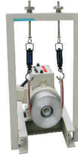
AC Motors with standard Mechanical loading arrangement
