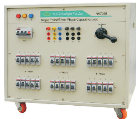
Single and Three Phase Capacitive Load
