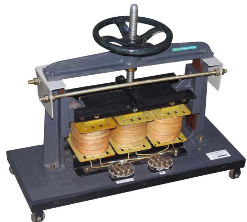
Three Phase Inductive Load
