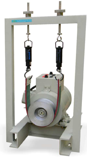
DC Motors with standard Mechanical loading arrangement
