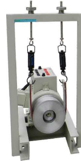
AC Motors with standard Mechanical loading arrangement
