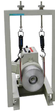
AC Motors with standard Mechanical loading arrangement
