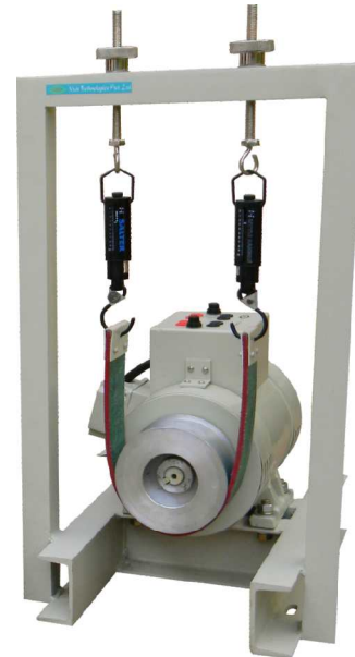
DC Motors with standard Mechanical loading arrangement
