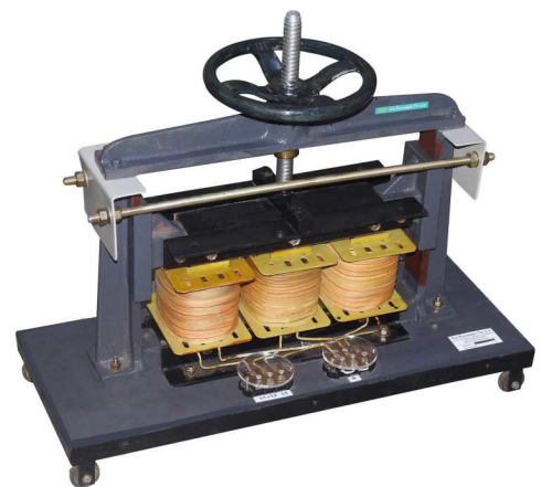
Three Phase Inductive Load
