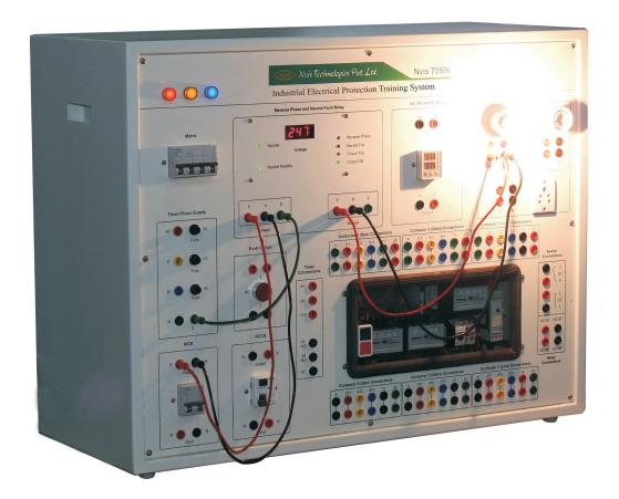
A relay is an automatic device which senses an abnormal condition of electrical circuit and closes its contacts. These contacts in turn close and complete the circuit breaker trip coil and make the circuit breaker disconnect the faulty portion of the electrical circuit from rest of the healthy circuit. Nvis 7059I Industrial electrical protection training system is provided to demonstrate the operating principle of over current relay, over voltage relay, under voltage relay and earth fault relay.
