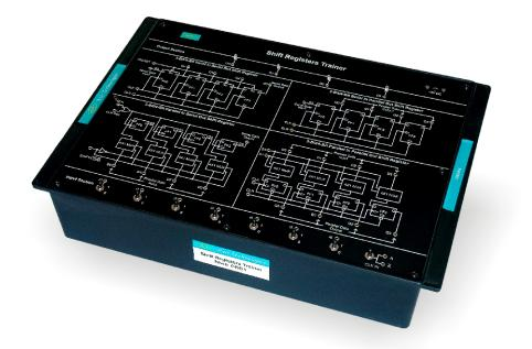
**Nvis 6561 Shift Registers Trainer** is a compact, ready to use digital electronics experiment board. This training product has been designed specifically for students to study all the four types of 3-bit and 4-bit shift registers on a single board and verify their truth tables.
