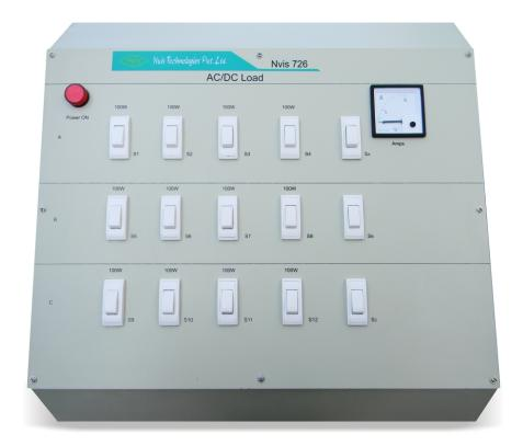
Nvis 726 AC/DC Load is an important device in all the Electrical laboratories. One can connect a load upto 1.2KW using this product. The device comes with On Board Switches, so that one can vary the load as required, in steps of 100W. The product is designed so as to provide load for various experiments of Transformer, Motors, Generators etc.
