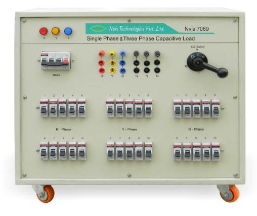
**Nvis 7069 Single Phase** & Three Phase Capacitive Load consists of three banks of switchable capacitors. These three banks can be used with Single Phase & Three Phase Systems. The load banks are used to verify the performance of power source. However real loads are unpredictable and random in value hence standard loads are used and this stimulates environment for testing power sources. The capacitive load bank provides a leading power factor.
