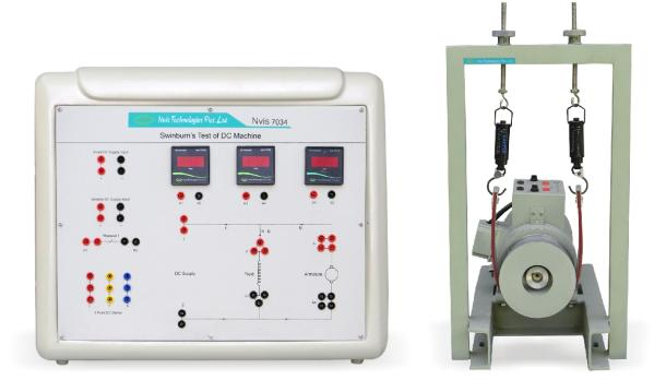
Nvis 7034 Swinburn's Test of DC Machine is an important training system for Electrical Laboratories. It can be aptly employed for understanding the fundamental concepts and functioning of DC Motor. Swinburn's Test is the method through which losses are measured separately and efficiency at any desired load can be predetermined.
