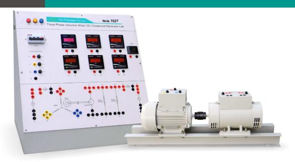
**Nvis 7027 Induction Motor Compound Generator Lab** is an adaptive training system for Electrical laboratories. It is designed to demonstrate the fundamental concepts of DC Compound Generator on different loading conditions. The diagrammatic representation is provided on the control panel so that students can make connections themselves. All protection circuits are inbuilt, so there is very less chance of fault or danger.
