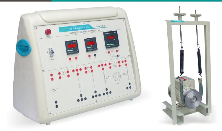
**Nvis 7015 Single Phase Induction Motor Lab** is an exclusive and attractive training system for the electrical laboratories. It provides complete learning concepts of Single Phase Capacitor Start Induction Motor. Separate terminals have been provided for main winding, starting winding and capacitor so that student can understand the significance of individual windings along with the role of capacitor in the motor in a simple manner.
