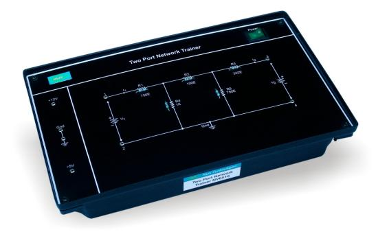
**Nvis 6516 Two Port Network Trainer** has been designed specifically for Two Port Network analysis. This is useful for students to study the operation and behavior of any two-port network under several operating conditions. The study of two-port network is very important as they form the building block of most electrical systems.
