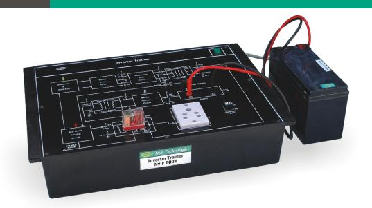
**Nvis 6001 Inverter Trainer** is a versatile training System for Laboratories. It is designed such that all the basics of Inverter can be easily understood. This training system provides understanding about conversion of DC into AC by PWM Technique. Different blocks are explained like charging of battery, DC to AC conversion, AC mains sensing circuit, etc. Nvis 6001 is also provided with fault switches to develop the troubleshooting practice.
