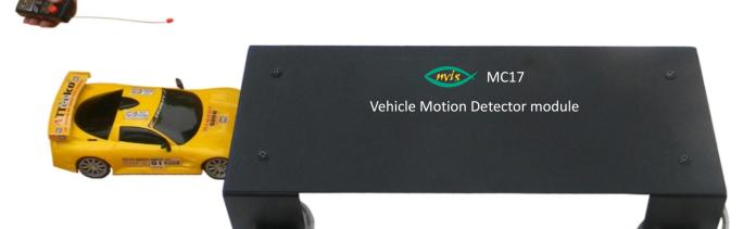
Nvis Technologies Vehicle motion detector module, MC17 is an extension for Nvis Microcontroller development platforms. The object is to have a clear understanding of how to measure the speed of vehicle using Microcontroller. Vehicle motion detector module. MC17 has input and output terminals for connection of external real world applications.
