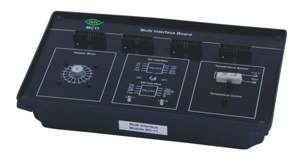
**Nvis Technologies Multi interface module MC11** is an extension module for Nvis Microcontroller development platforms. The object is to have a clear understanding of how input peripherals are interfaced and controlled with Microcontroller. MC11 has been designed to have a clear understanding of how Stepper Motor is interfaced and controlled with Microcontroller. It also gives a clear understanding of SPI and I<sup>2</sup>C interface bus for data transfer.
