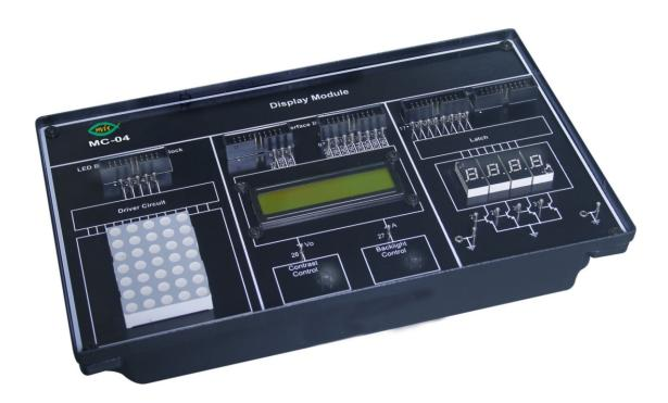
**Display module MC04** is a learning platform to study the working of displays used for industrial applications. MC04 has been designed to demonstrate the applications of Nvis Microcontroller development platforms. The object is to connect and program a Microcontroller to display data and monitoring. Contrast and backlight control are provided on the module.
